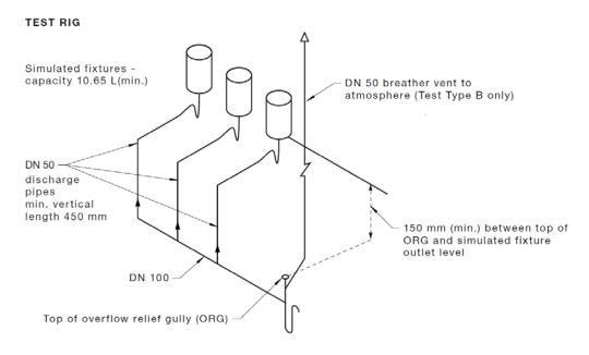
FIGURE D1 TEST RIG TO SIMULATE FIXTURES DISCHARGING INTO AN ORG
