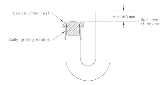
FIGURE C1 TYPICAL OVERFLOW-RELIEF TEST SET-UP
